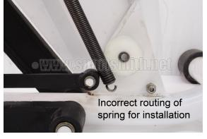
You must insert the end of the spring into the pulley groove
